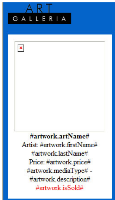
Figure 50. Variables don't get processed properly just because you put number signs (#) around them.
